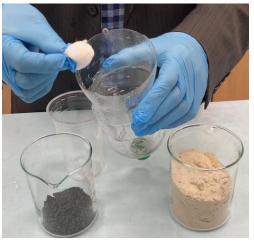
Step 4 – Empty half the sand in the bottle as shown in picture on the right. Shake the bottle to get the sand to settle onto the wool balls. Then pour the layer of activated charcoal on top of the sand. Make sure the layer of activated has a consistent depth. Pout the remainder of the sand over the activated charcoal.
