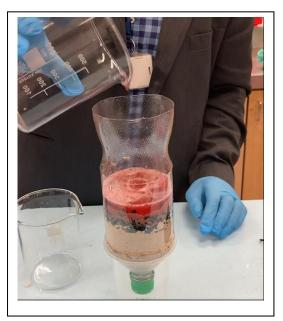
Step 9 – Pour the rest of the contaminated water, that you have been supplied with, through the water purifier and collect the purified water in the cup.
